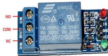
Gambar 5. Modul Relay 1 Channel
