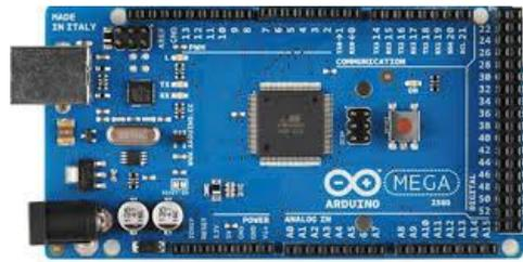
Gambar 2. Arduino Mega 2560
