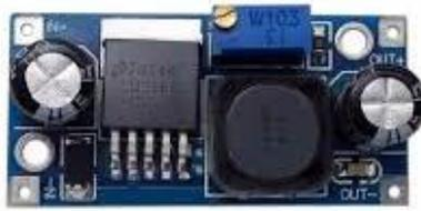
Gambar 8. Modul DC-DC *step down* LM2596
